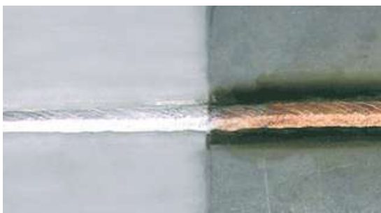
Before and after pickling. Avesta Pickling Paste 101 – for brush pickling in all positions.
